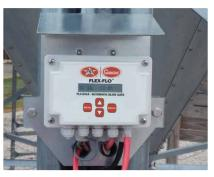
**REMOTE OPERATION** Ability to operate slide gates at the tank or remotely inside the barn for increased bio-security.
